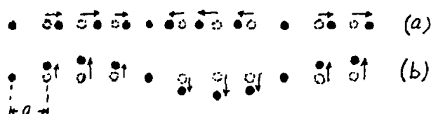
Longitudinal (a) and transverse (b) modes with wavelength 8a in a one-dimensional mono-atomic crystal. The arrows show the displacements from the equilibrium positions.
